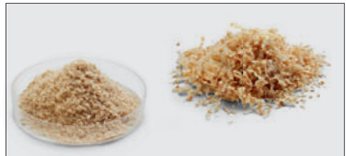
Medium-hard and fibrous materials like wood can be easily comminuted with the cutting rotor.
